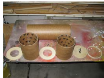
Altimeter Bay Components
