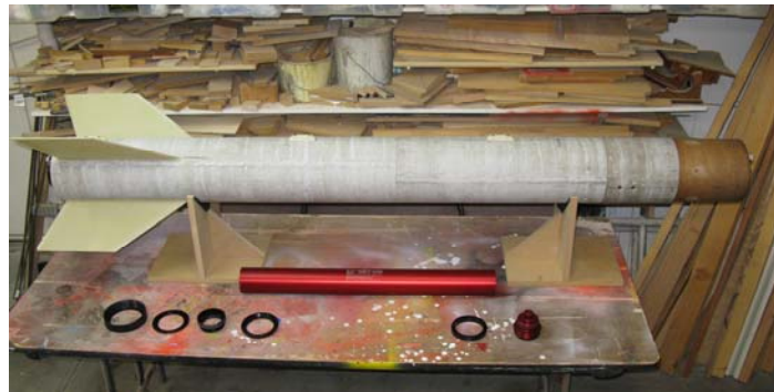
Dr Rocket 75/6400 Motor Casing and Adapters
